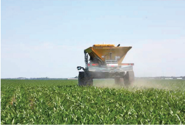
Figure 48. Variable rate fertilizer applicator used to establish plots illustrated in Figure 42 (Reetz Agronomics).
