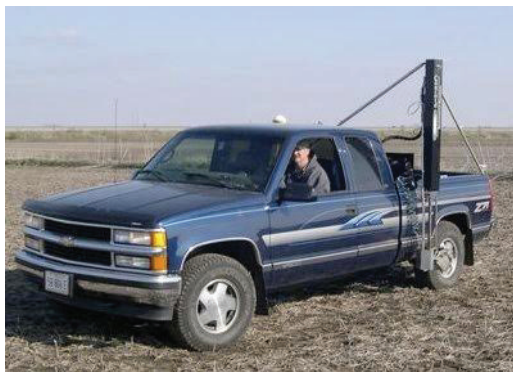
Figure 20. Hydraulic samplers mounted on a pickup truck or ATV help to reduce the workload in collecting soil samples, especially for deep sampling (CropSmith).
