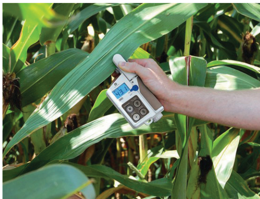
Figure 26. The SPAD chlorophyll meter is a tool for estimating "greenness" of leaves, an indicator of relative N content (Spectrum Technologies).
