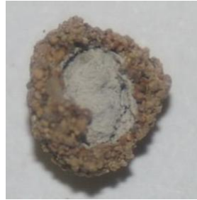
Microphotograph of P fertilizer granule incubated for 4 wks in a calcareous soil
