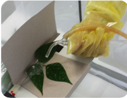
Fig 3 - AFTER TREATMENTS, RAINFASTNESS (30 mm \pm 2.5 – 15 minutes) WAS SIMULATED BY USING A MANUAL SPRAYING
