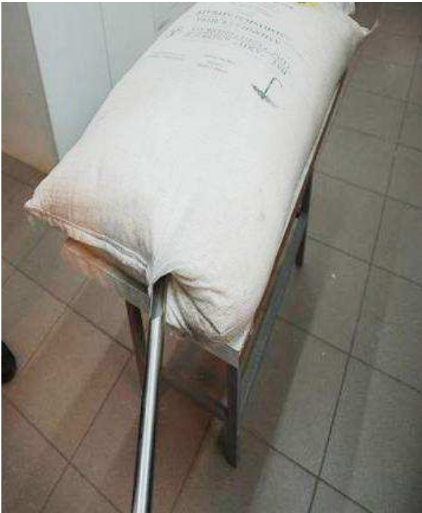
Figure 12. Collecting an increment; single tube trier.
