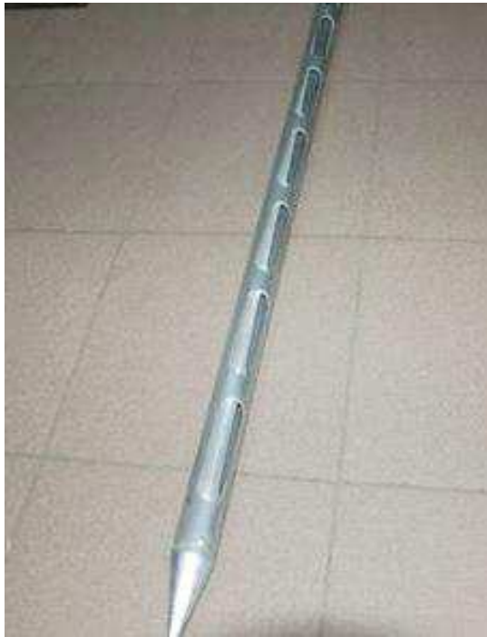
Figure 6. A double tube trier (SPL-03).
