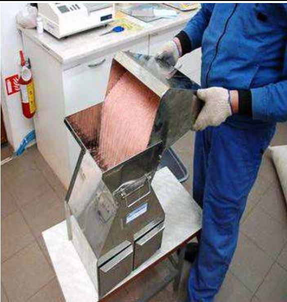
Figure 16. Dividing a sample with an enclosed riffle with a feed chute and fed by a feed pan that is as wide as the riffle.
