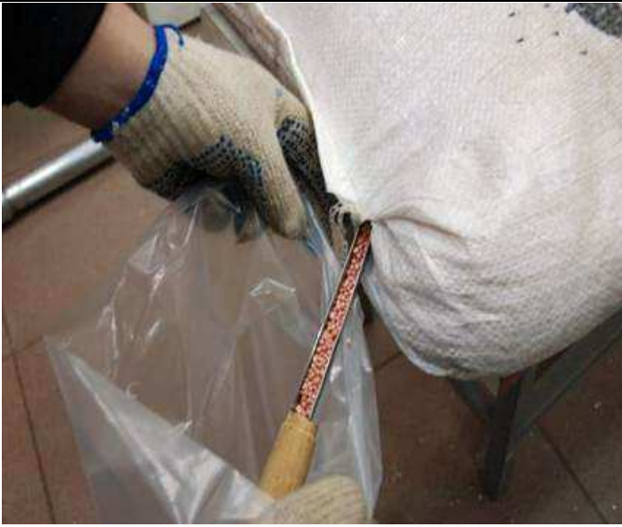
Figure 10. Collecting an increment; sampling spear.
