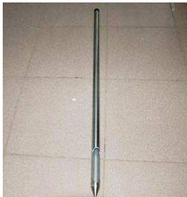
Figure 5. A single tube trier (SPL-02).
