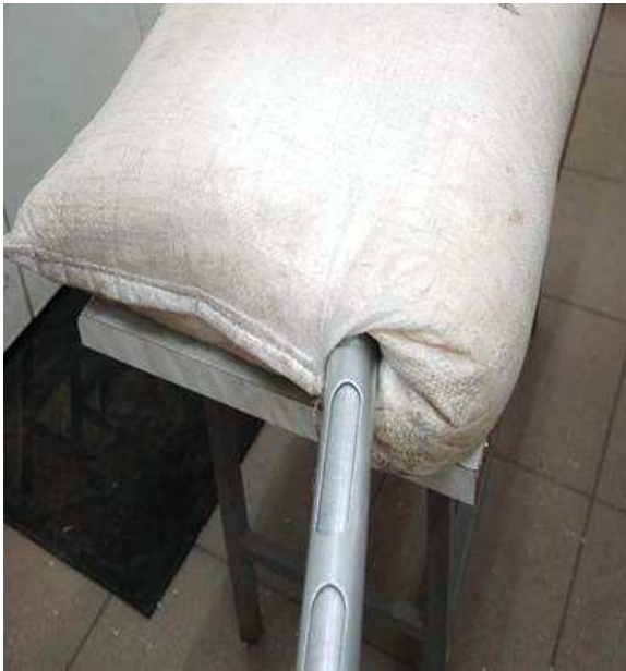
Figure 14. Collecting an increment; double tube trier.
