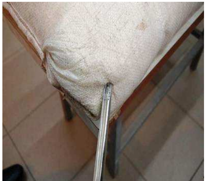
Figure 9. Sampling diagonally across a horizontal bag; single tube trier.
