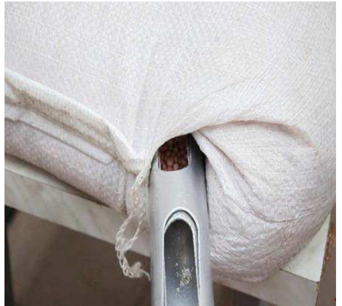
Figure 15. Collecting an increment; double tube trier.
