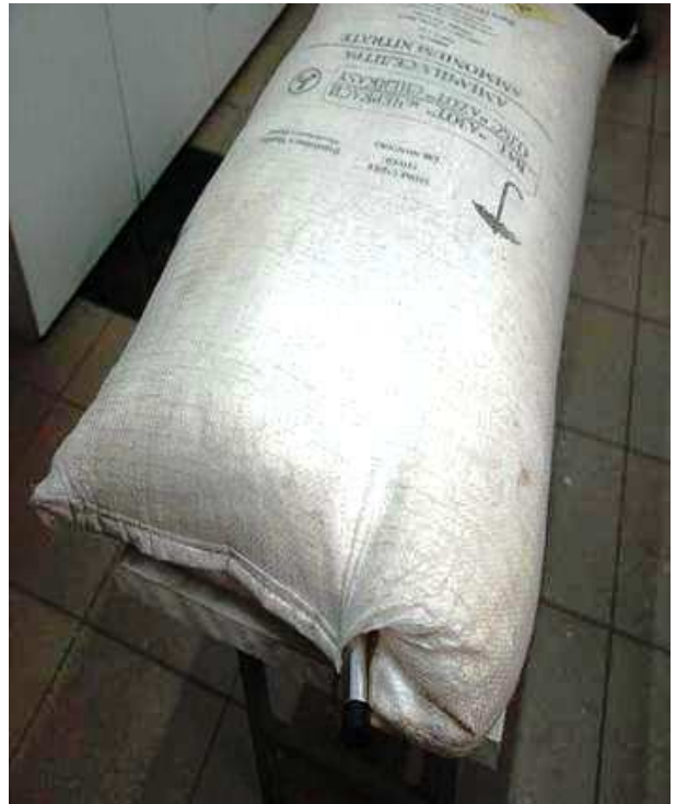
Figure 13. Collecting an increment; single tube trier.
