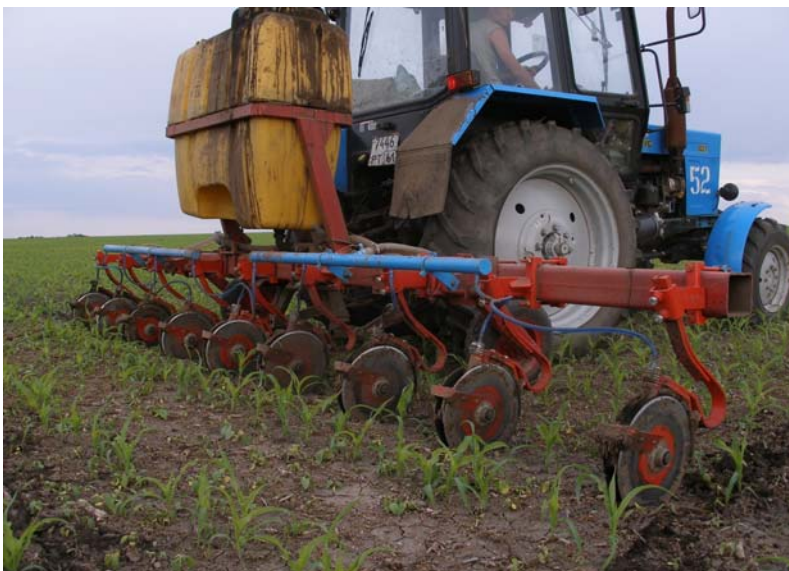
Root feeding of cultivated crops with liquid nitrogen fertilizer (UAN 32) with the use of disc coulters.
