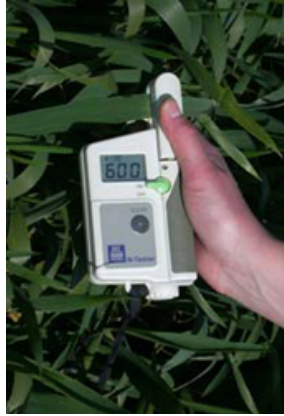
Chlorophyll meter system on winter wheat to assess the N quantity for the last application
