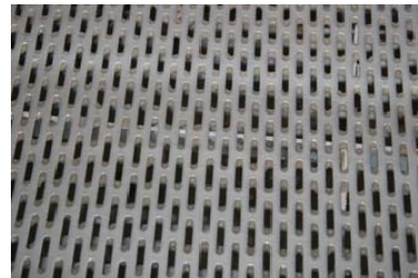
Fig.-17 Tendency of scale formation on the Filter perforated sheets of Aqaba PA plant, (After linking up the digester)
