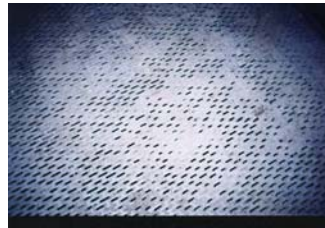
Fig.-7 Tendency of scale formation on the filter Perforated sheets of Aqaba PA plant (Before Linking up the digester)
