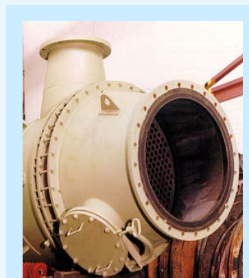
Rubber lined top header: A manhole is possible on large diameters.
