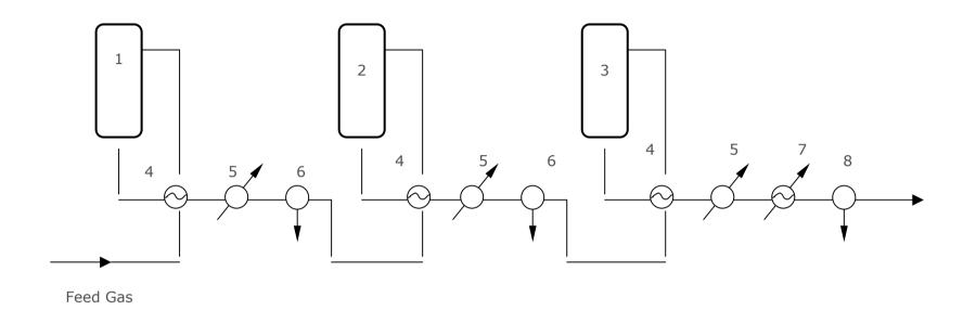
1, Alcohol tower 2, Alcohol tower 3, Alkylation tower 4, Gas-Gas heat exchanger 5, Water Cooler 6, Gas-Liquid Separator 7, Ammonia Chiller 8, Gas-Liquid Separator
