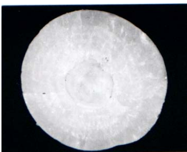
Figure 4. Section of Urea-based MAP Granule(4.0mm).
