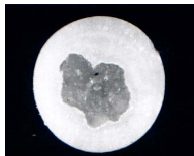
Figure 5. Section of Urea-based DAP Granule(3.6mm).
