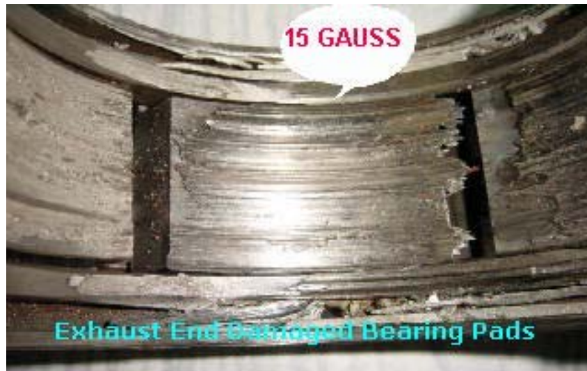
Photograph 2 Damaged Bearing Pads
