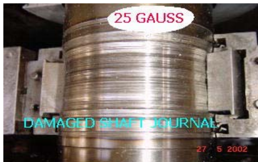
Photograph 1 Damaged Shaft Journal
