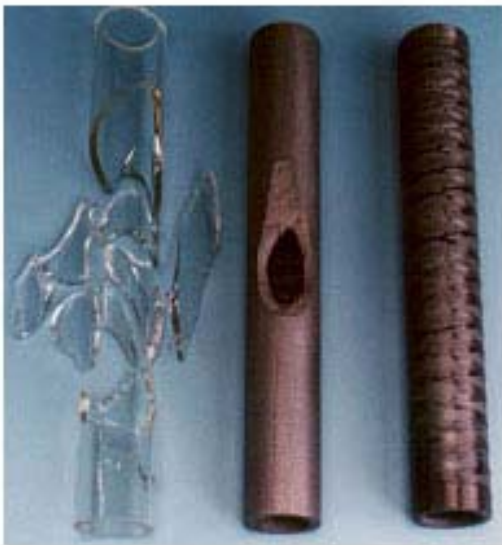
Fracture behavior of glass-, standard graphite tube and fiber reinforced graphite tube
