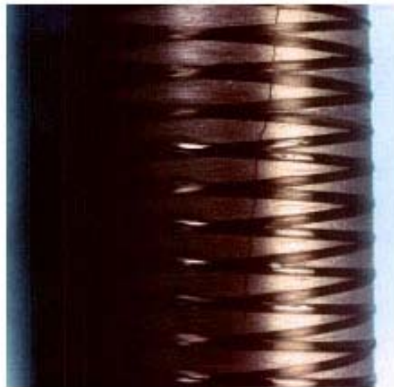
Fracture behavior of glass-, standard graphite tube and fiber reinforced graphite tube
