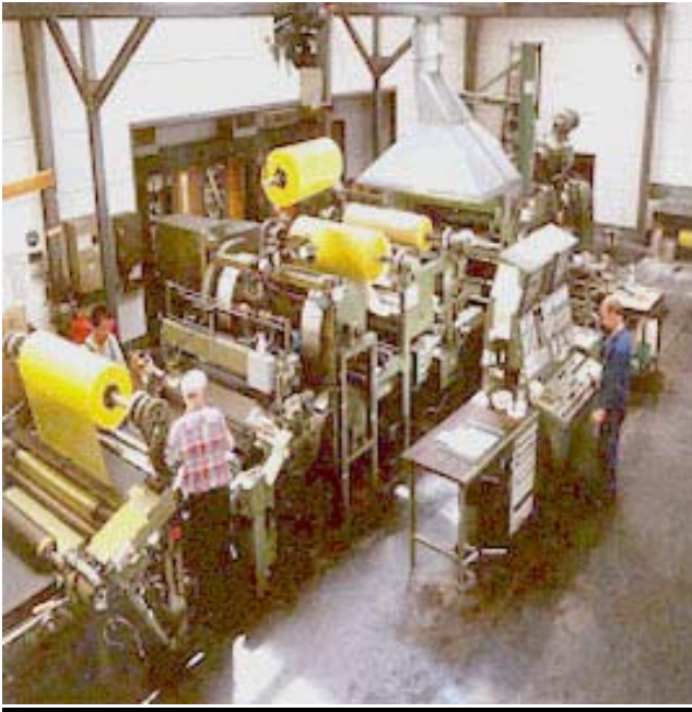
Roller head extruder for rubber sheets
