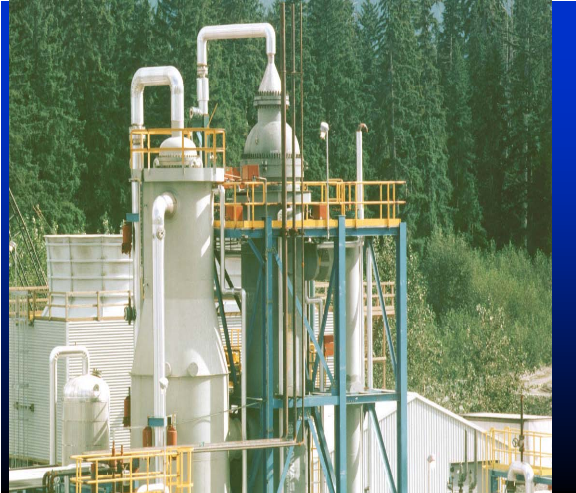
Fig.1: KRES at plant in Canada, with autothermal reformer on the left and reforming exchanger on the right.
