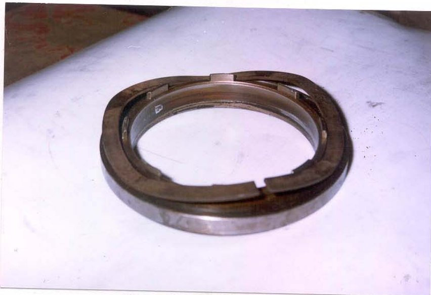
SEAL ASSEMBLY IN RIGHT WAY (Edge of the Leaf spring NOT resting on seal ring face)
