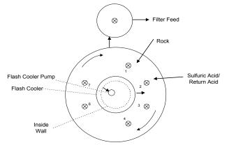
mounted in the center of the reactor. Cooled slurry overflows from the flash cooler between agitators 2 and 3. Rock is added near the No. 1 agitator and sulfuric acid and return acid near the No 2 agitator. Slurry overflows from the reactor between agitators 7 and 1 to a filter feed tank.
