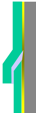
Water absorption behind the rubber. Bonding force is weakened
