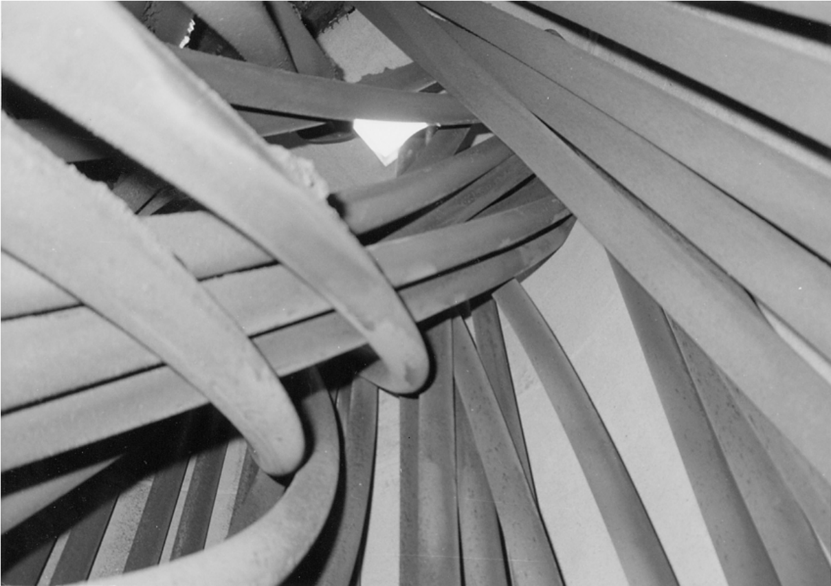
PHOTOGRAPH N°1 : TUBES IN RADIANT SECTION OF 103-B FOUND ENTANGLED DUE TO OVERHEATING
