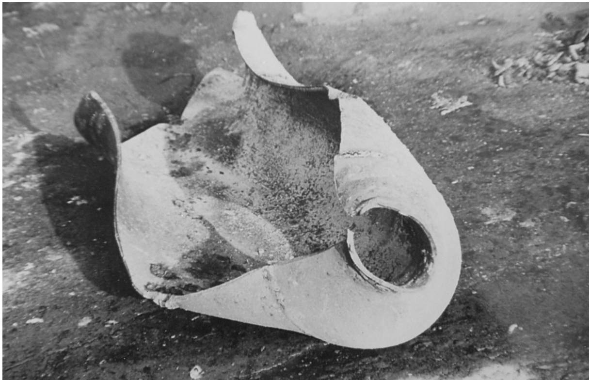
PHOTOGRAPH N°6 : SHEARED OFF TAIL PIPE OF RV-156-C
