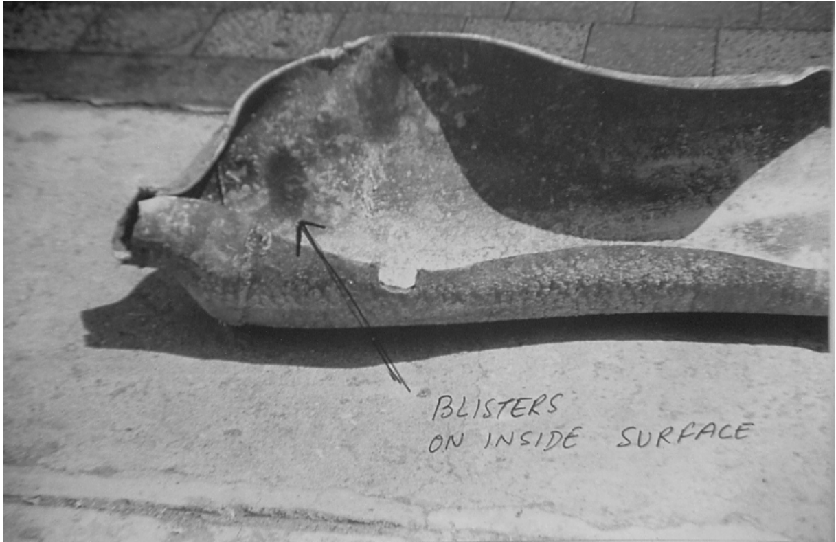
PHOTOGRAPH N°5 : SHEARED OFF TAIL PIPE OF RV-156-C
