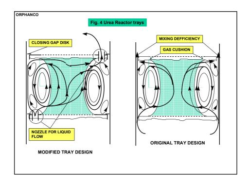
• By applying the above two main modifications the CO<sub>2</sub> conversion in the reactor could be maintained at 60 to 61% at the new capacity of 2850 MTD (see Figure 5)
