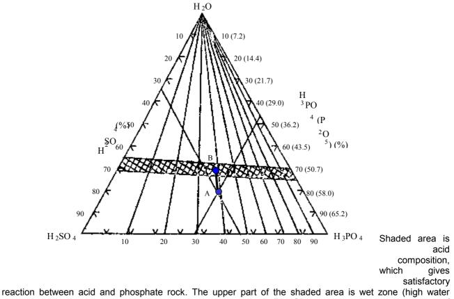
reaction between acid and phosphate rock. The upper part of the shaded area is wet zone (high water content), while the lower point is dry zone (low water content). The SP-36 process has a composition of  $35.1\% P_2O_5$  and  $34.5\% H_2SO_4$ , and if this is drawn on the triangle diagram, it will be found at point A (dry zone). To reach the shaded area, water must be injected, so point A will move to point B.
