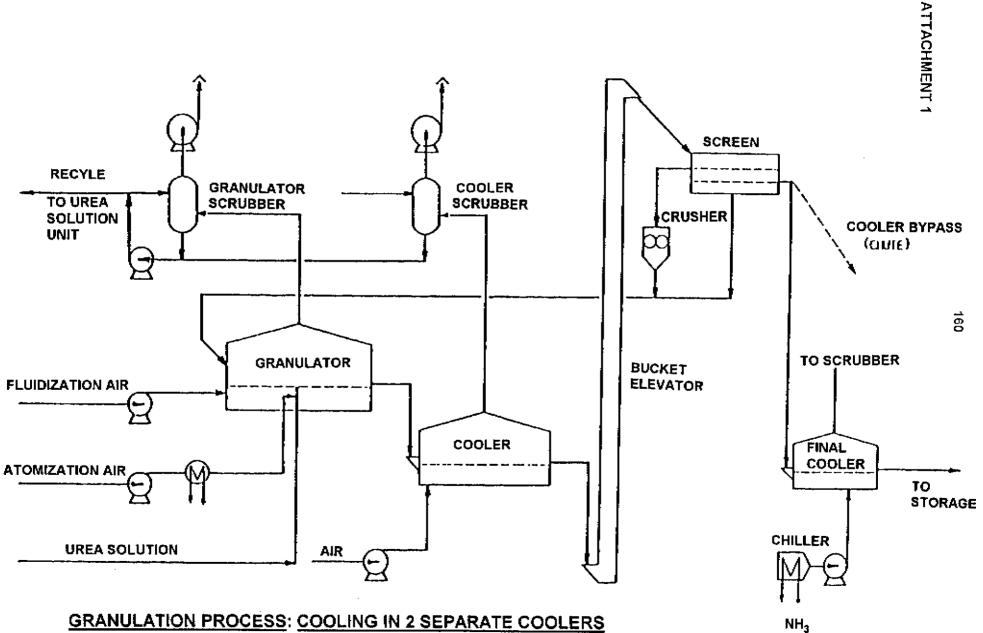
**GRANULATION PROCESS: COOLING IN 2 SEPARATE COOLERS**
