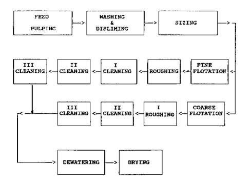
Figure 4: Washing and disliming flowsheet
