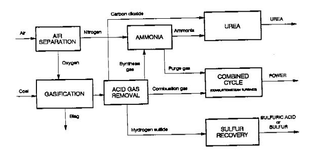
Figure 1 IOCO/FERTILIZER COPRODUCTION PROCESS CONCEPT
