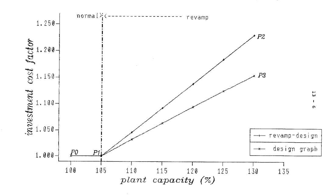
The sequence is also directly proportional to absolute equipment costs and represents the necessary steps for uprating the equipment to the new plant capacity. Modifications of the compressor set cause the highest expense, whereas modifications of the steam system can be achieved at relatively low cost. The given reserve of 20% for the steam system does not mean 20% more in steam production but is related only to the heat flux.
