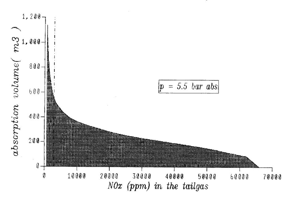
installed equipment, certainly with respect to justifiable economic expense. With reference to the details on the absorption volume pointed out, the following example should explain in which way an optimum can be determined between an extended absorption section and a selective abatement system. The result of this investigation yields the maximum nitrous gas concentration in the tailgas at which an extended absorption can be operated economically in combination with a selective abatement system.
