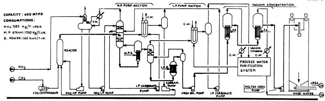
FLOW- SHEET OF THE ABOVE PLANT RETROFITTED ACCORDING TO I.D.R. MONTEDISON TECHNOLOGY (PROPOSED)
