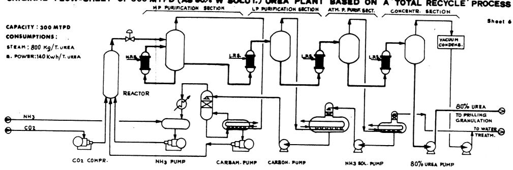
FLOW- SHEET OF ABOVE PLANT REVAMPED TO 650 MTPD (AS 80% W. SOLUT.) BY I.D.R. MONTEDISON TECHNOLOGY (PROPOSED)
