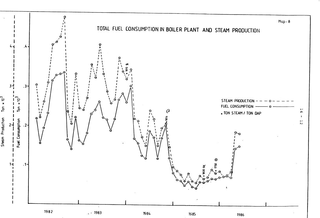
Adding fixed losses in the boiler plant and steam distribution lines as also inside the plant, we obtained the total steam requirement of 875 what remotes the 1 300 kg steam per tonne DAP allocated budget, before 1983, which became 800 in 1985 by decision of the Production Department.
