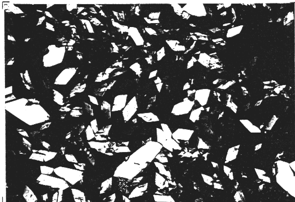
Figure 7 - Gypsum crystals obtained with Montaline (neg. 7196) SP/CV A1 surface-active agent (100x)
