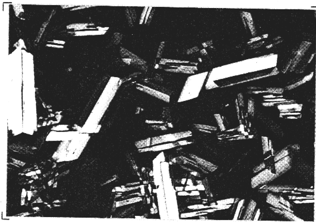
Figure 8 - Gypsum crystals obtained with Montaline (neg. 7270) SP/CV Al surface-active agent and kiesel g uhr (100x)
