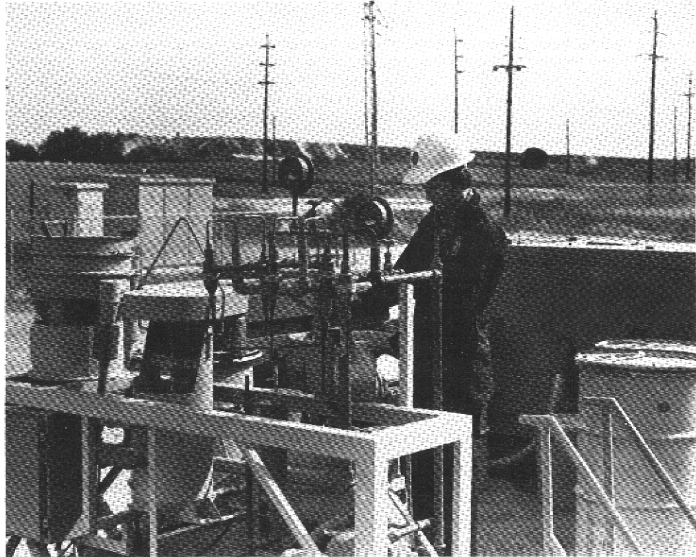
Figure 3. Two-stage cyclone unit for onsite classification of phosphate slimes at six operating phosphate washers.
