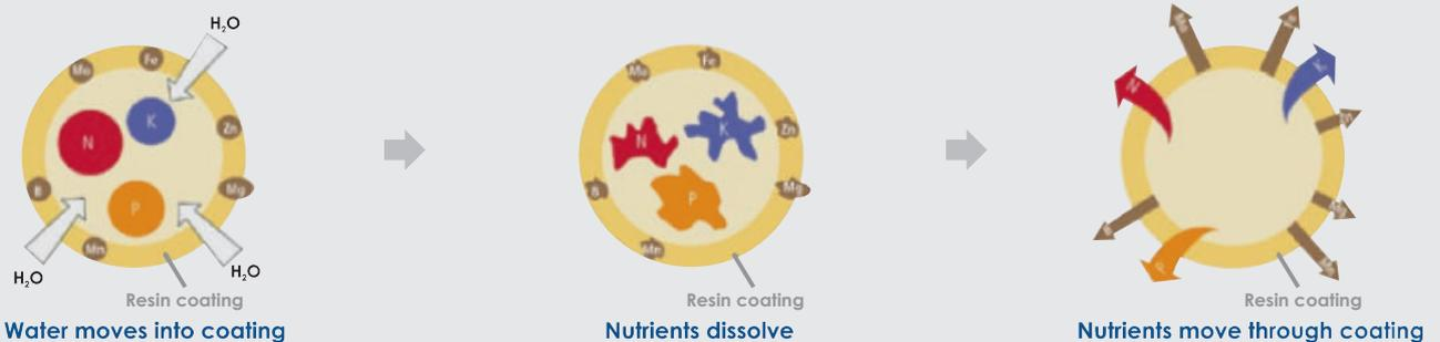
Mode of action of a coated/encapsulated controlled-release fertilizer
