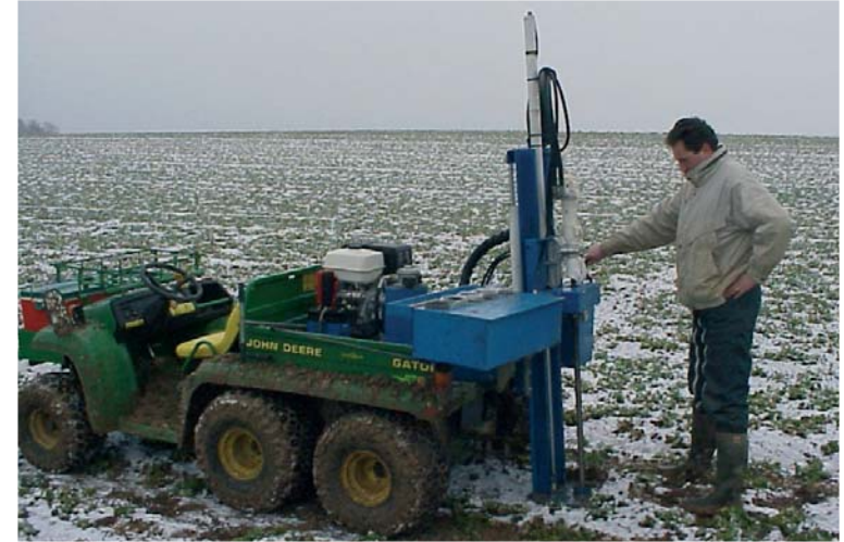
Picture 7. Soil sampling (Credit: INRA - LDAR Laon)
