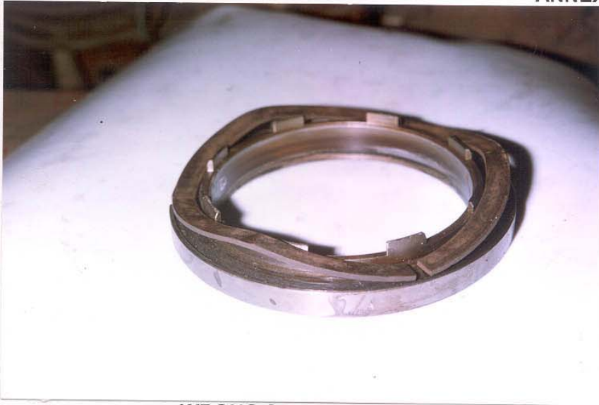
WRONG SEAL ASSEMBLY (Edge of the Leaf spring resting on seal ring face)
