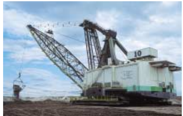
Surface mining of phosphate rock with dragline, Florida - Cargill Fertilizers Inc., USA
