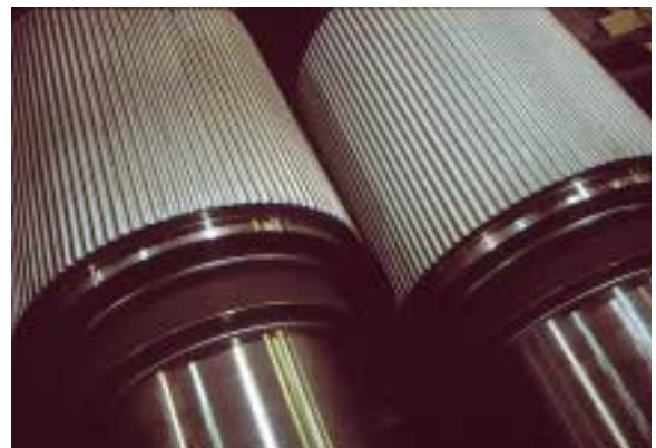
Potash compaction rollers - Potash Corporation of Saskatchewan (PCS), Canada
