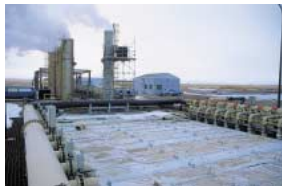
Heating potash brine prior to injection - Potash Corporation of Saskatchewan (PCS), Patience Lake, Canada
