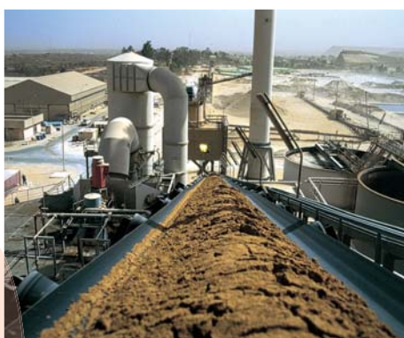
Feeding the phosphoric acid reactor with phosphate rock. Darou, Sénégal.
